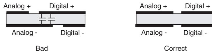
Power planes are designed using the same rules as ground planes. Keep the analog supply plane entirely under the analog ground plane, see on [Figure 2-5: Correct](#). This gives an analog supply plane over the analog ground plane and a digital supply plane over the digital ground plane. In this case, it could not cause unwanted capacitance between the two planes.
