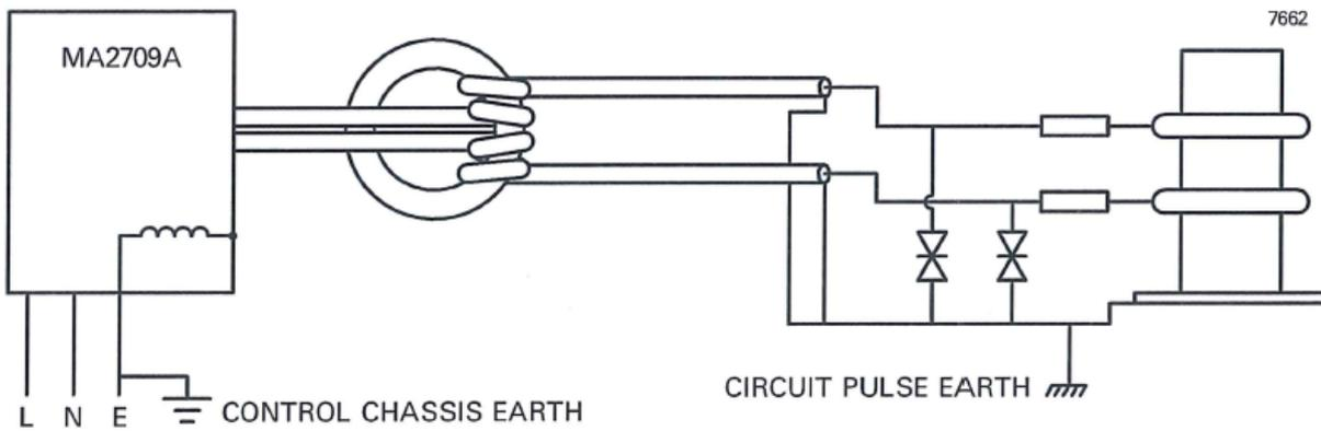
Fig.2 MA2709A mounted close to the thyatron discharge circuit
