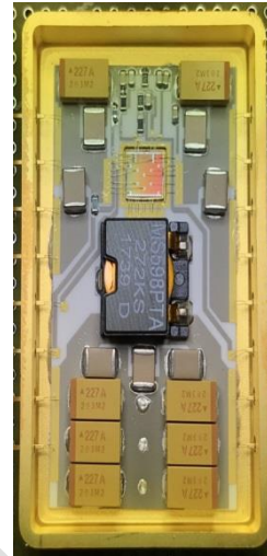
16-pin HTCC Hermetic Flat Pack Package
