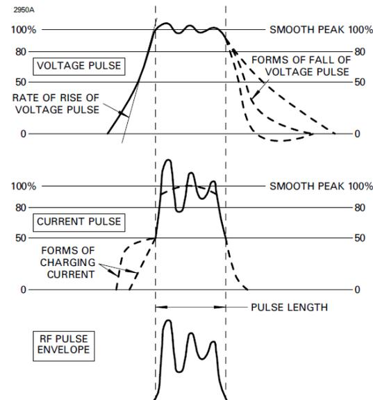
Fig.5 Pulse waveforms
