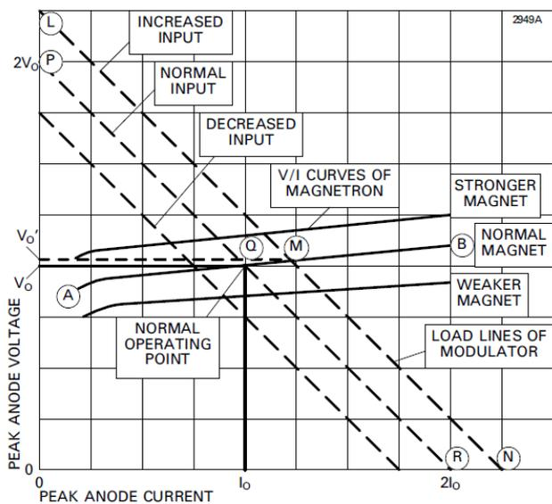
Fig.3 Line-type modulator characteristics
