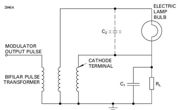
**Fig.1** Heater dissipation test circuit
