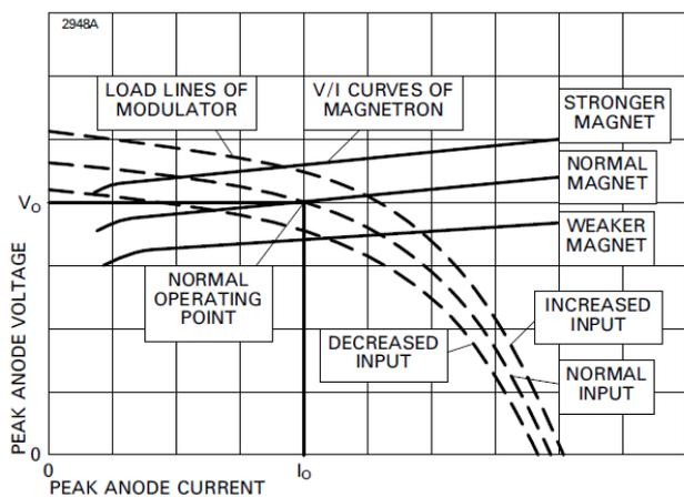
Fig.4 Hard tube modulator characteristics
