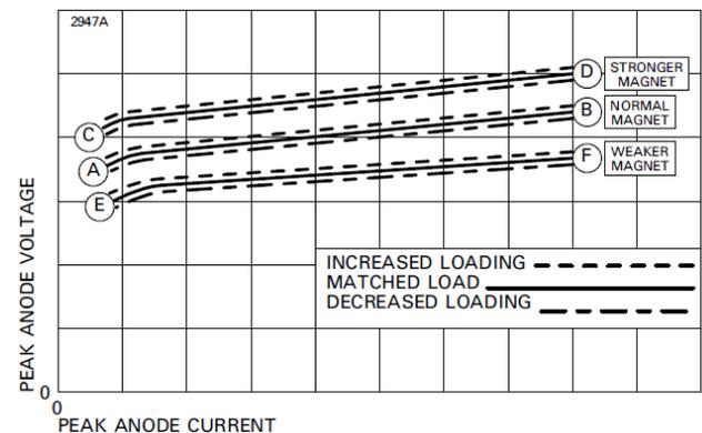
Fig.2 Magnetron impedance characteristics
