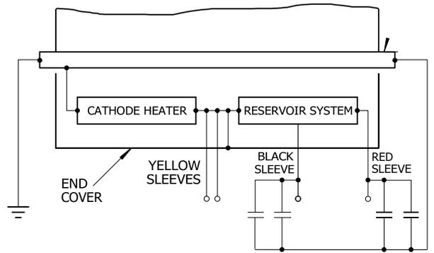
Fig. 2 CX1937X base connections
