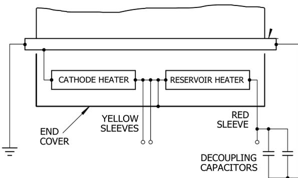
Fig. 1 CX1937 base connections
