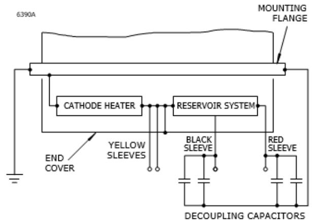
Fig. 2 CX1547X base connections
