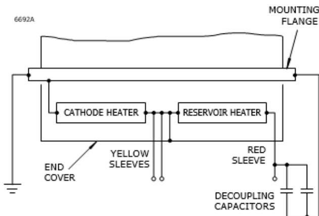
Fig. 1 CX1547 base connections
