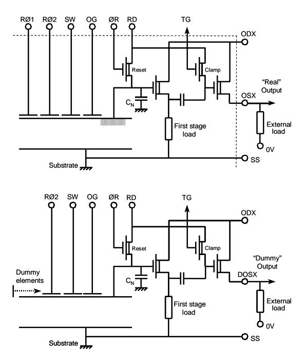
The first stage load of each output (real or dummy) draws a quiescent current of approximately 0.2 mA via SS.
