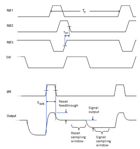
Alternative clocking with RØ3 clocked with SW is also acceptable if independent connection to SW is not available or binning on to SW is not required.
