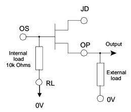
The output impedance is now 100  $\Omega$  and the within-package dissipation is typically 50 mW per amplifier.
