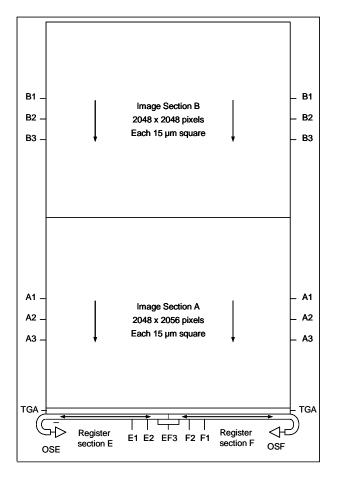
Device structure looking down onto the photo-sensitive surface
