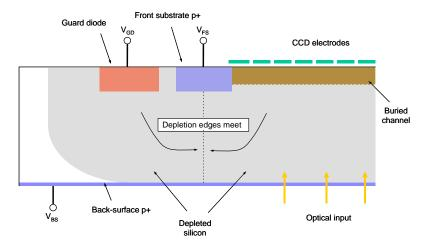
With correct bias conditions the depletion regions from the CCD channel and the guard diode merge to block the conductive path, rather like the operation of a JFET, as shown above. If incorrect, then there is a direct resistive path between the front and back contacts and excessive currents can flow, as shown below.
