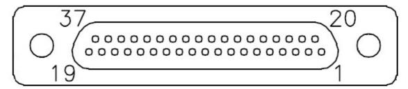
This numbering applies to all connectors. The connector is a Glenair 37P micro D type.
