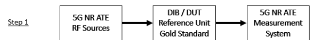
Figure 1a. Simplified Block Diagram: Manual Reference Plane Calibration Utilizing Gold Standard Reference Unit
