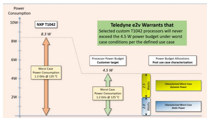
Figure 1: T1042 processor worst case power specification versus customer's target use case.
