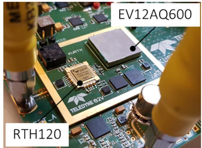
Figure 2 - Photo of initial prototype FEB on its carrier board
