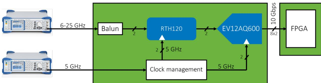
Figure 1 - FEB test evaluation set up showing key active devices
