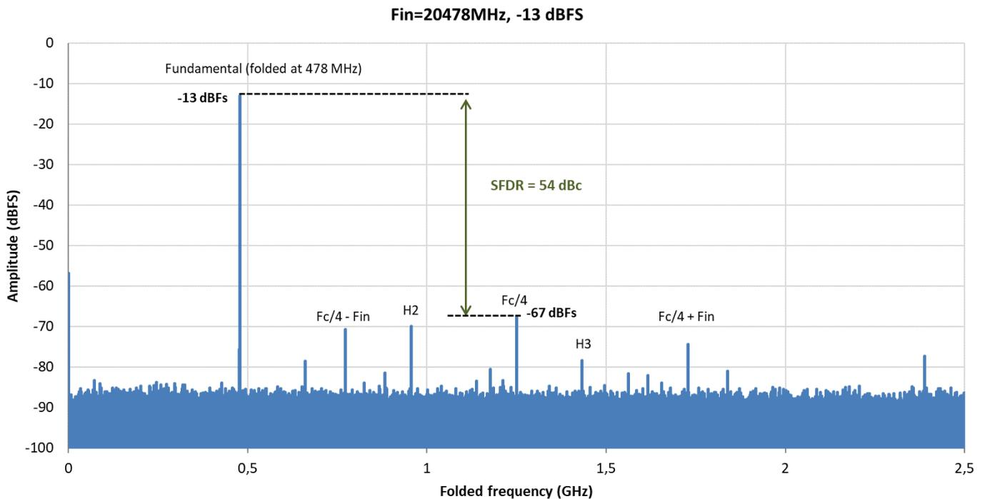
Figure 8 - Spectral plot of 20.478 GHz tone down converted to baseband with the experimental FEB
