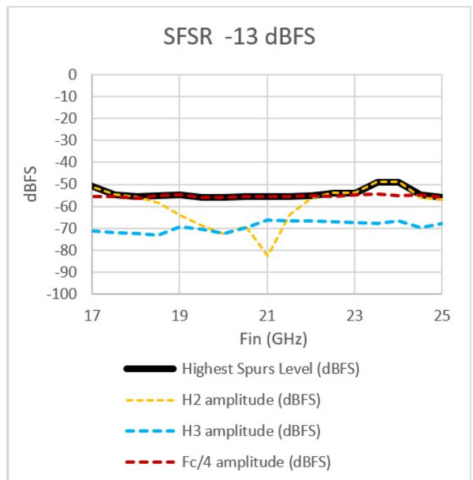
Figure 4 - The baseline FEB performance at two signal powers (SFDR swept from 17 to 25 GHz)
