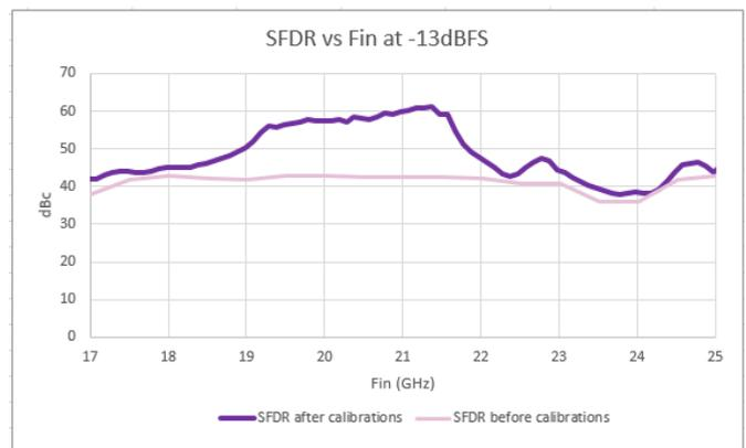
Figure 7 - K-band SFDR pre- and post calibration
