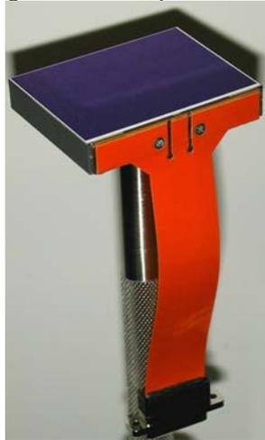
Figure 2: - A CCD91-72. Note that a handling tool can also be seen in the photograph.
