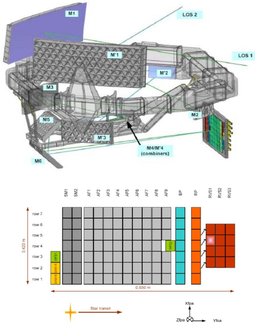
Figure 1: - The Gaia Telescope arrangement (top) and the focal plane layout (bottom) (Images courtesy of EADS Astrium)
