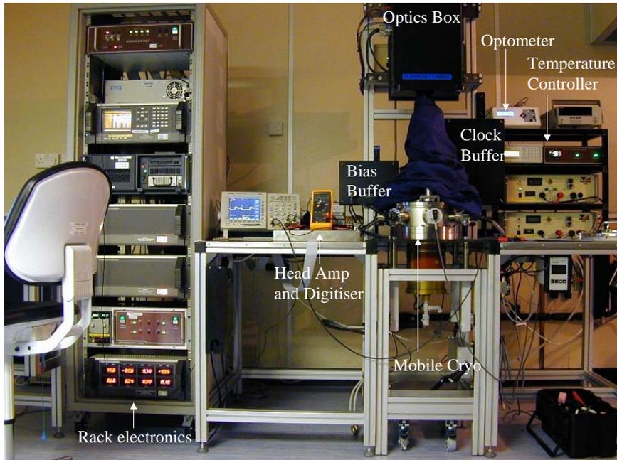
Figure 4: - A photo of a Gaia Test Camera
