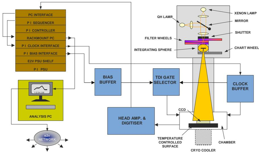
Figure 3: - A schematic of a Gaia Test Camera
