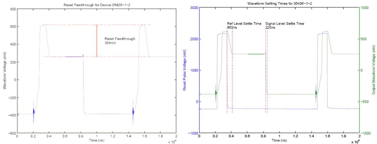
Figure 10: - Examples of waveform measurements using a virtual oscilloscope and automatic software analysis
