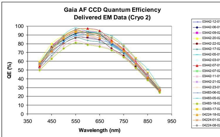
Figure 5: - Measured QE curves for the 20 AF devices delivered in the TD phase.
