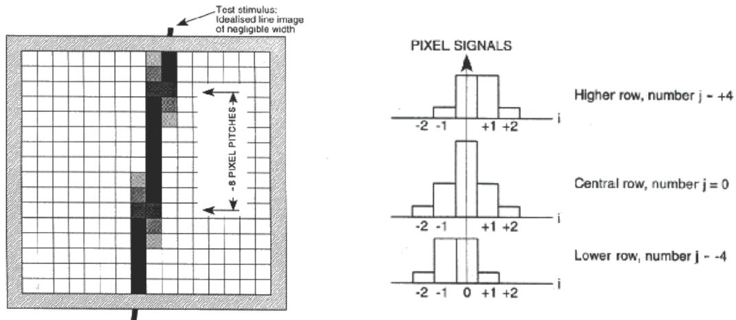
Figure 7: - Schematics of MTF Slit Image (left) and signal in top, middle and bottom row of the angled slit image (right)
