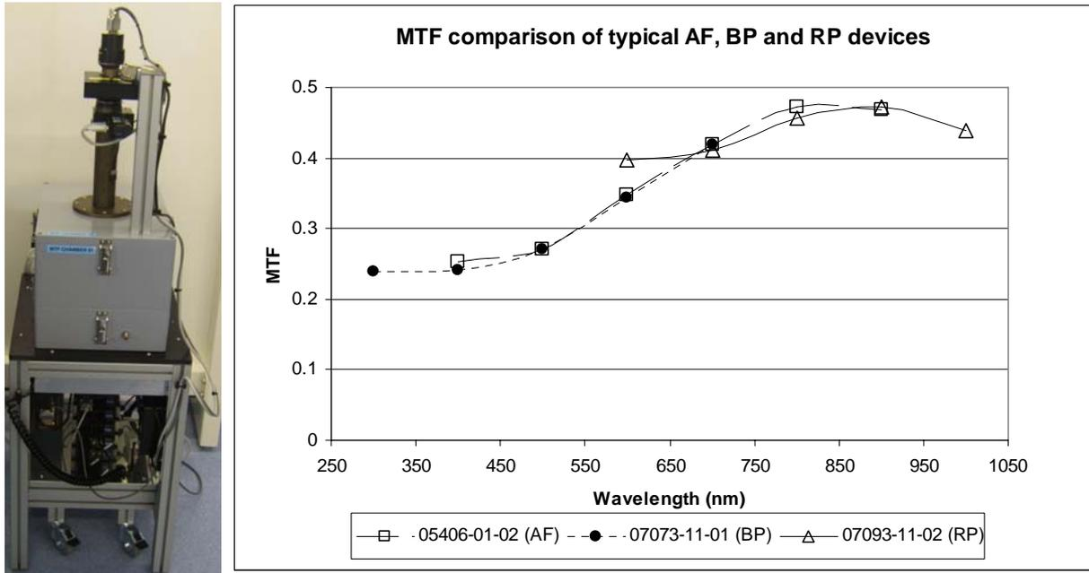
Figure 8: - A photo of the new automated MTF chamber (left) and MTF data (right) for a typical AF, BP, RP CCD91-72 from the Flight phase measured in the along track, small pixel dimension (10um) direction. MTF across track, in the dimension of the larger pixel dimension (30um), is typically 0.45 to 0.55 for all device types.
