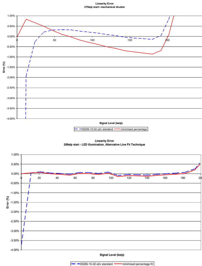
Figure 9: - Linearity plots over a signal range of 200 to 190,000 electrons using shuttered tungsten lamp (top) and LED illumination (bottom). The dashed lines are using standard line fitting where the absolute residuals are minimised, the solid lines are where the percentage residuals have been minimised in the line fitting. Both plots use data from the same device.
