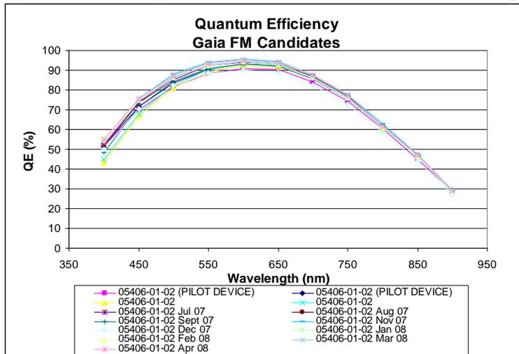
Figure 6: - Multiple QE measurements of the Flight Phase Control Device taken between February 2007 and April 2008. Note this curve includes measurements from several different cryos and different cameras. The spread at the blue end of the spectrum shows the inherent variation of the sensitivity of the device surface, e.g. with molecular absorption.
