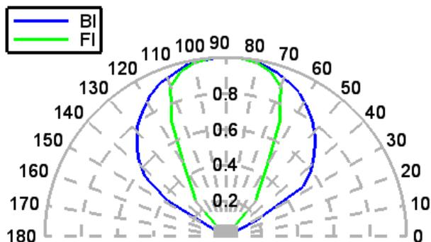
Figure 4 – Normalized Angular response
