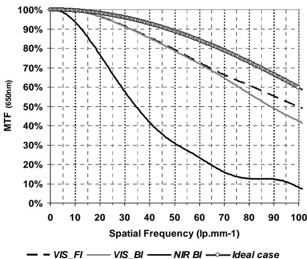
Figure 6 – Modulation Transfer function (650 nm)
