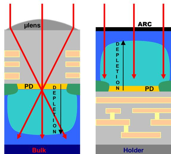
Figure 1 – Back illumination principle
