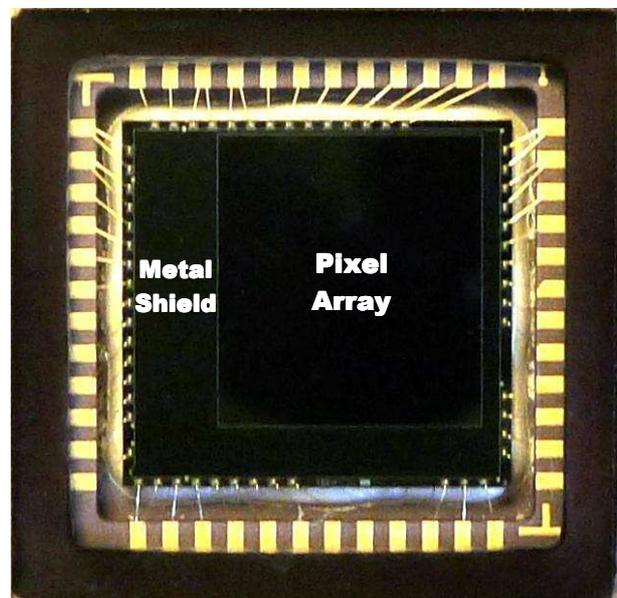
Figure 3 – Micrograph of BI chip
