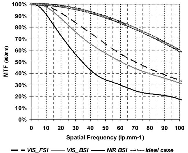
Figure 7 – Modulation Transfer function (900 nm)
