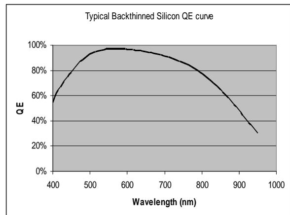
Fig.3. Typical Back-thinned Silicon QE curve.
