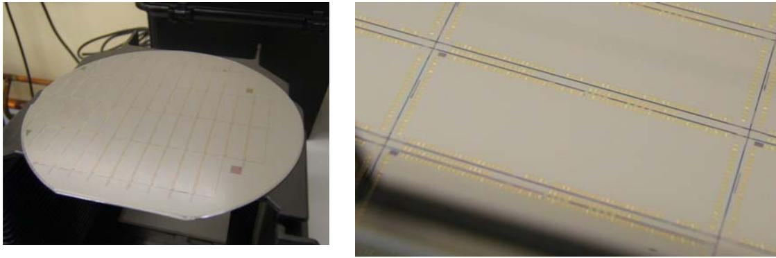
Fig.5. Backthinned Hyperspectral Wafer
