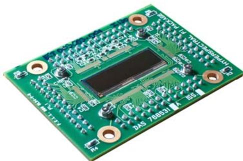
Fig. 6 Packaged Hyperspectral Imager
