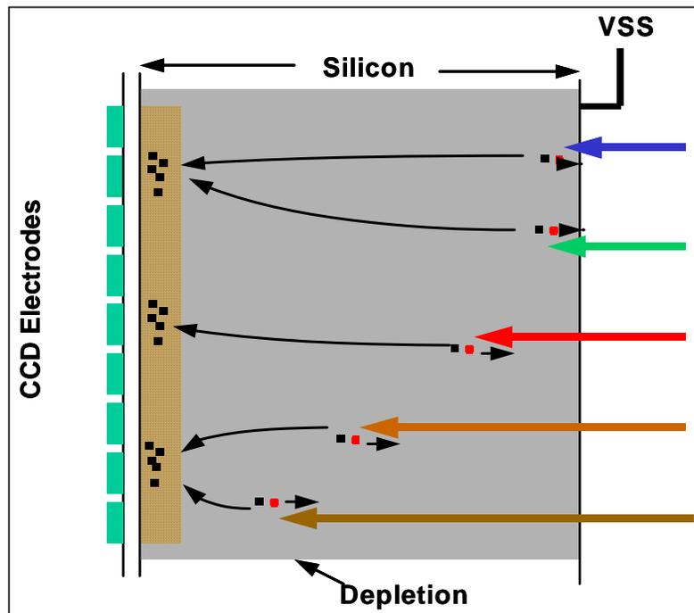
➤ Various modifications of the device structure are required to support the voltage (VSS) of up to -100V that is necessary at the back surface.
