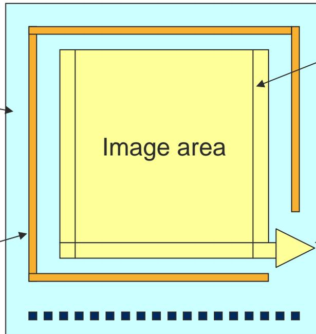
Dump columns are incorporated to provide a clean edge to the image region
