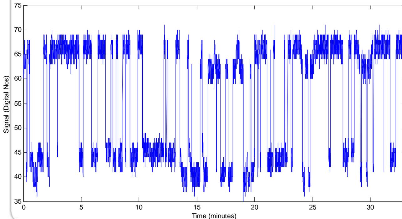
➤ RTS dark signal image from a CMOS sensor after proton radiation. Thanks to Ben Dryer and Prof. Andrew Holland for the CEI, The Open University.
