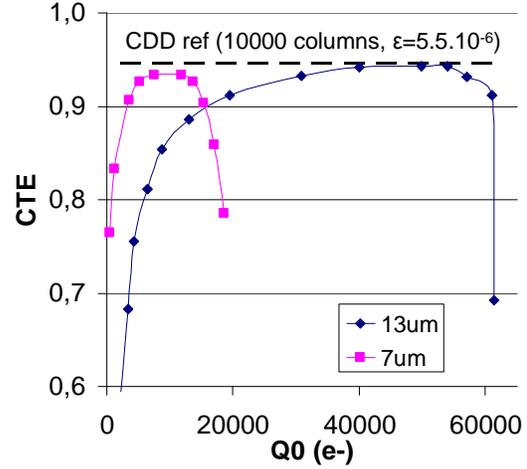
Figure 12. Measurement of the CTE of our TDI array (40 lines with column readout) as a function of the number of injected charges (Q0) for the 13um and 7um structure. A equivalent CCD performance with register readout is also added.
