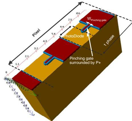
Figure 1. Innovative pixel architecture for charge transfer (shown here for 2 phases per pixel).
