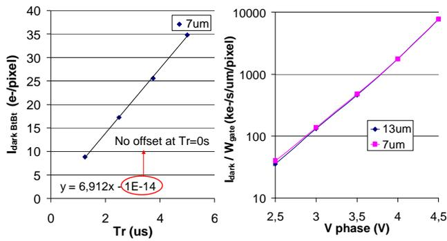
Figure 8. (Left) Measurement of the dark current offset as a function of the ON time of the transfer gates ( $T_r$ ) for the 7 $\mu\text{m}$  device. (Right) The dark current offset is measured as a function of the phase bias normalized with respect to the gate width for 7 $\mu\text{m}$  and 13 $\mu\text{m}$  ( $T_{\text{int}}=14\mu\text{s}$ ).
