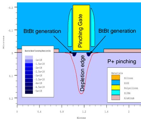
Figure 9. (Left) TCAD simulation of the BtBt dark current offset due to the P+ pinching implantation ( $T_r=2.5\mu\text{s}$ , 7 $\mu\text{m}$  structure). (Right) Output structure for  $V_{\text{phase}}=5\text{V}$  showing the localisation of the BtBt generation.
