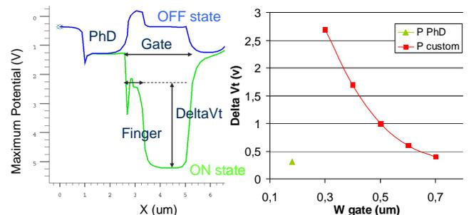
Figure 2. (Left) Maximum Potential simulated thanks to 3D TCAD along the pixel (extracted from a cutplane through the middle of the device). (right) Delta Vt as a function of the pinching gate width.
