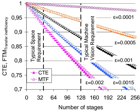
Figure 11. Calculation of the total CTE and the FTM at Nyquist due to the transfer inefficiency as a function of the number of TDI stages and the CTI. Open marks stand for the MTF and the filled marks stands for the CTE.
