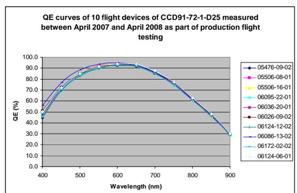
Figure 4: typical QE Curves for GAIA
