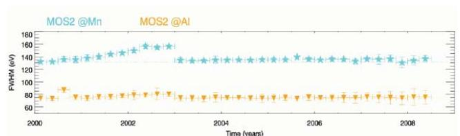
Figure 3: Energy resolution of EPIC cameras on XMM over nine years [2].
