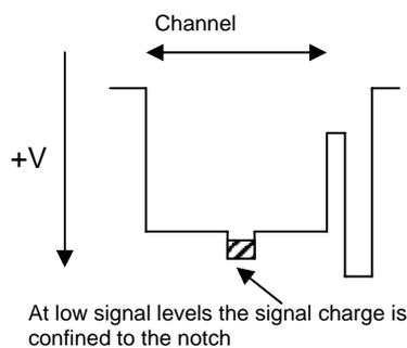
Figure 2: Potential cross section through a pixel with a notch
