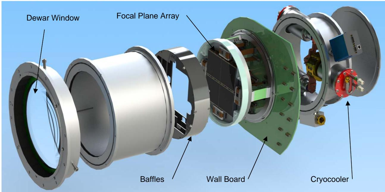
Figure 2. Exploded view of the KMTNet camera
