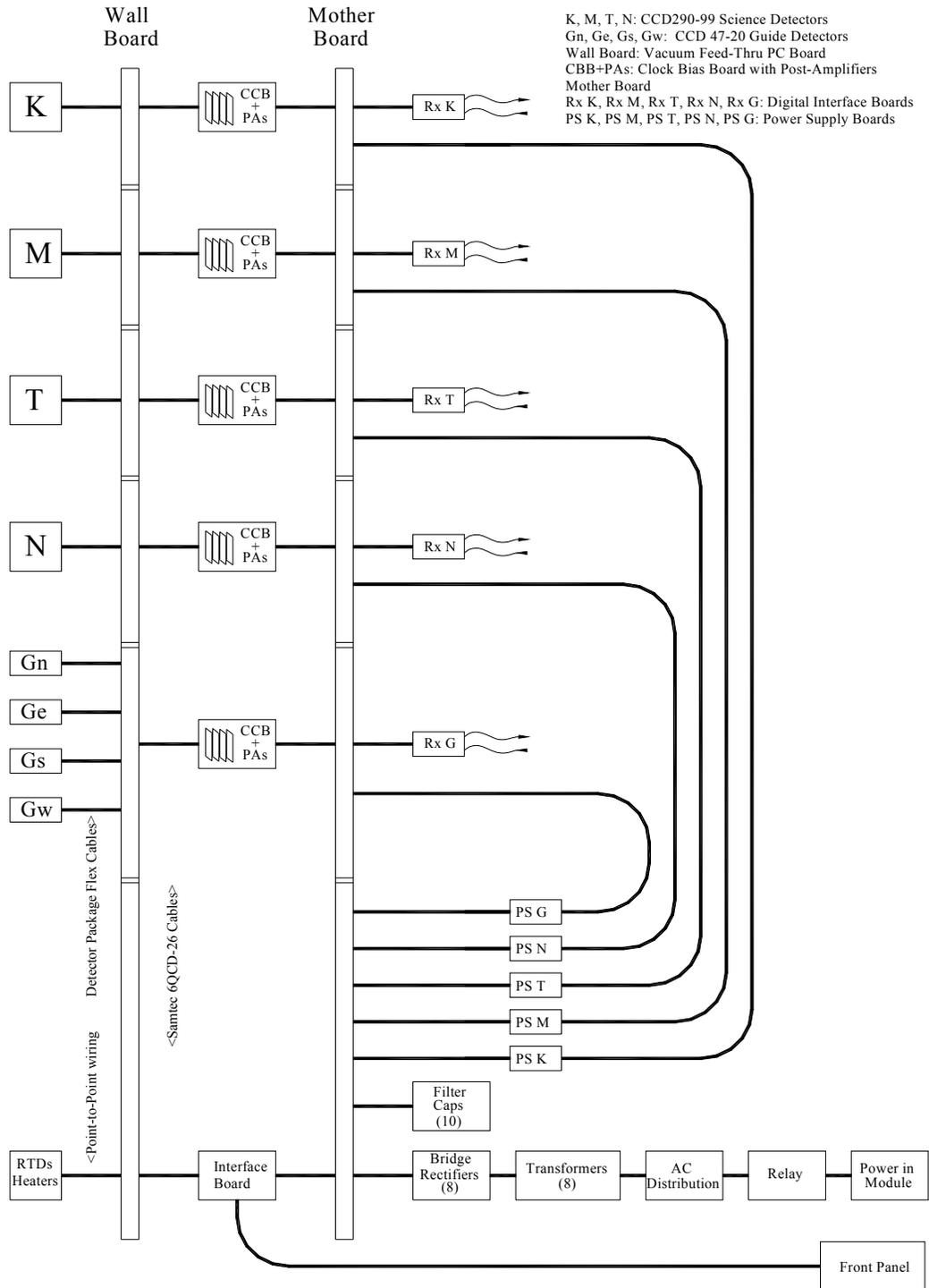
Figure 6. KMTNet HE System Diagram
