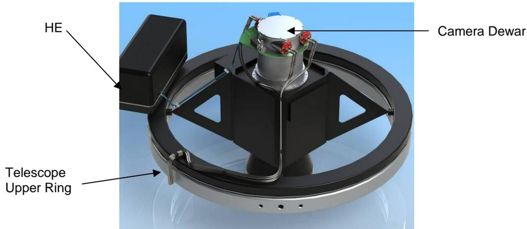
Figure 10. Isometric view of the telescope Upper Ring showing location of the Dewar and HE Box and cabling paths
