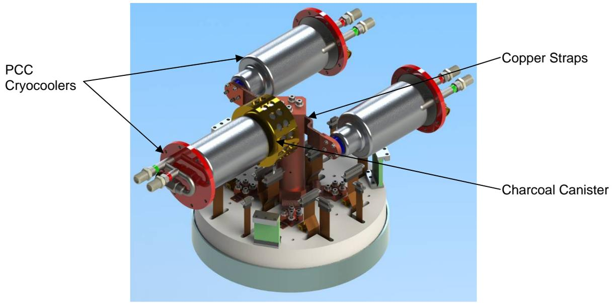
Figure 9. Detector Cooling system and cryosorption pump charcoal canister
