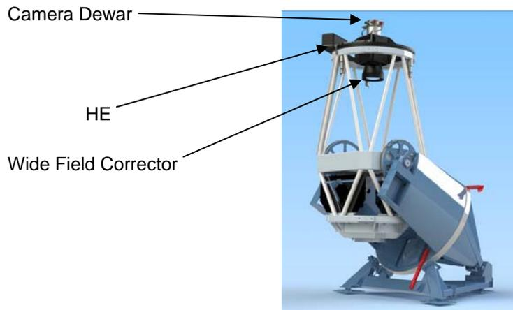
Figure 1. View of the telescope showing the location of the Camera and HE Box
