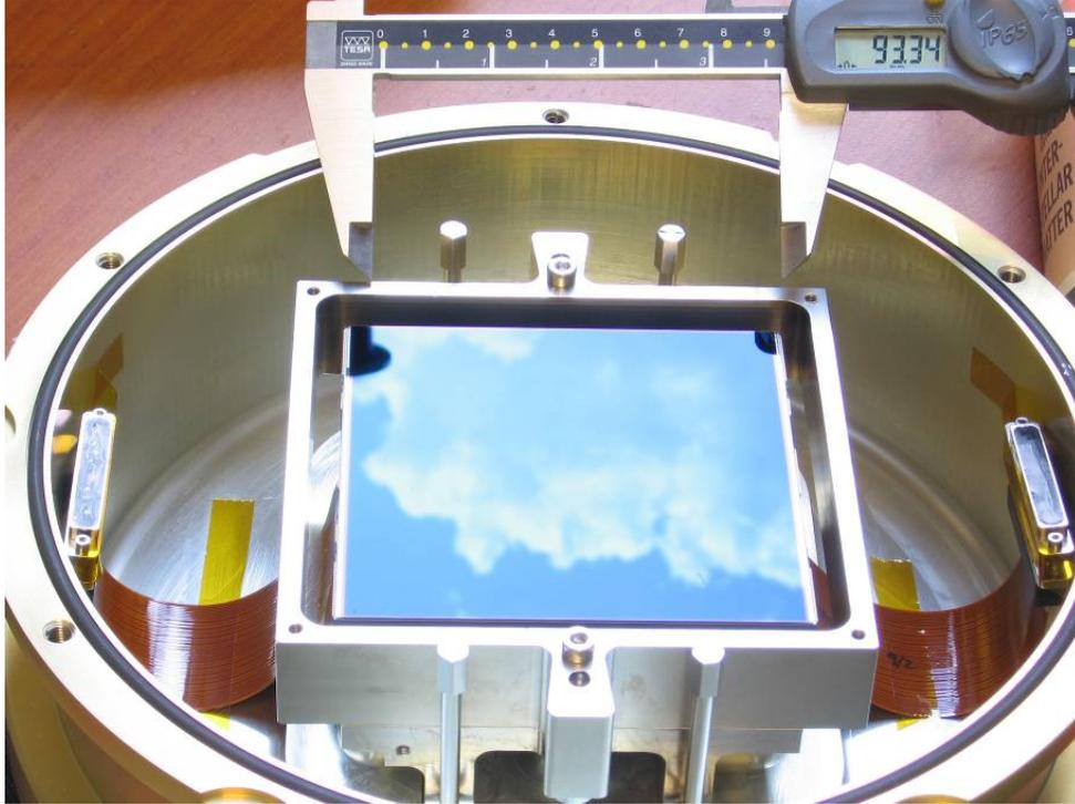
Figure 3. Image of a mechanical sample of the KMTNet science CCD. Flex cables are wrapped around in the shipping configuration with end connectors visible. The square box around the CCD is part of the shipping container.
