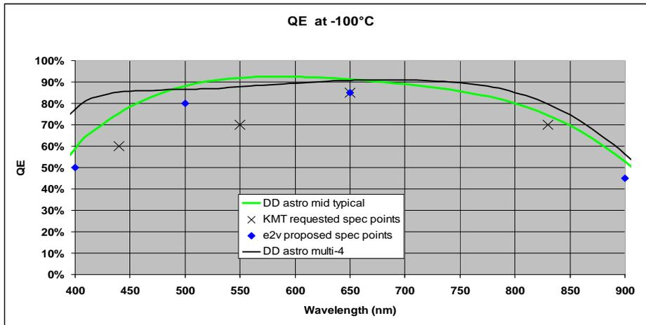
Figure 5. QE Curves of CCD290-99 Devices
