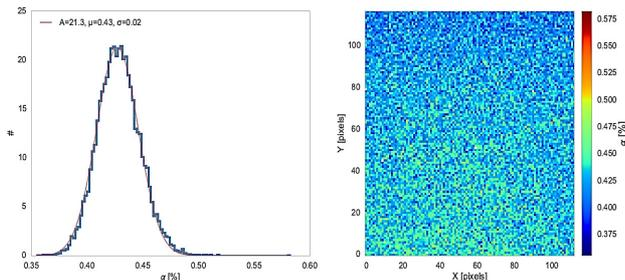
**Figure 9 – Measured distribution of  $\alpha$  on pixel-II**
