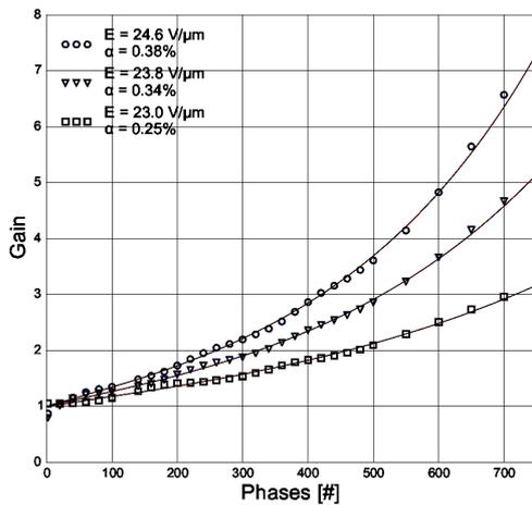
**Figure 8 – Measurement of EM gain on pixel-II**
