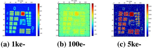
**Figure 11 – Pixel I - Images made under high illumination level (a), low illumination level without multiplication (b) low illumination level with 50x multiplication (c)**
