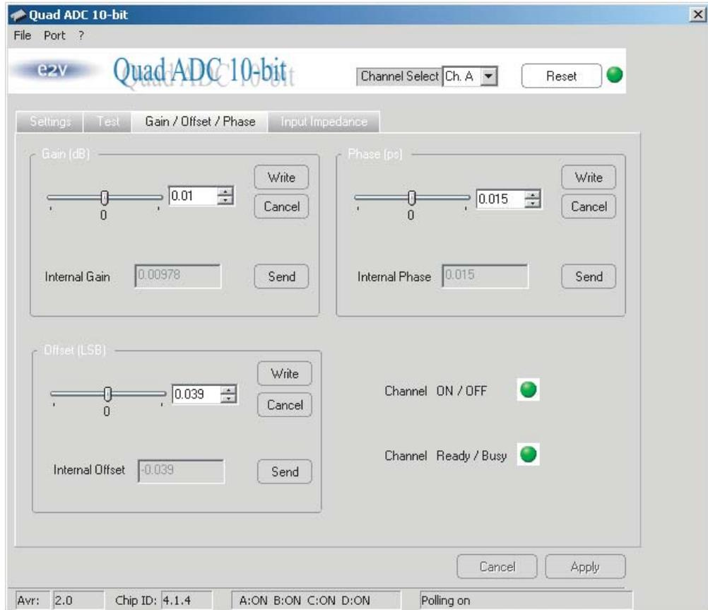
In the following example, you can see that the internal phase register is set to 0.015 and that the user wants the phase to be set to  $-15$  ps. In the second picture, the WRITE and SEND buttons have been pushed and the internal register shows the new entered value for the phase.
