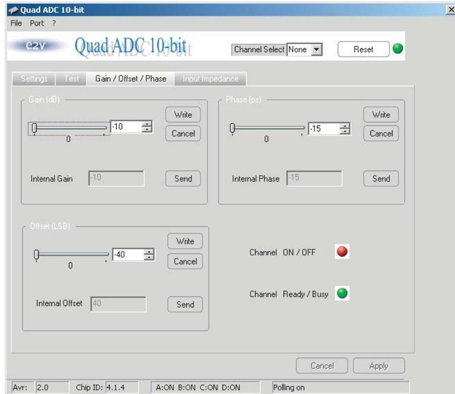
In this window, you can adjust the gain, offset and phase of the channel selected via the "channel select" button on the top right of the user interface.
