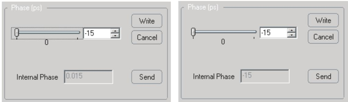
The iterative technique for calibrating the phase was described previously. Based on a reference phase for one channel the phase of the adjacent channels is adjusted so that the interleaving spurs decrease.
